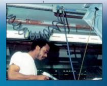
Trolleys running overhead on the aluminium pipework supporting and feeding pneumatic tools.
