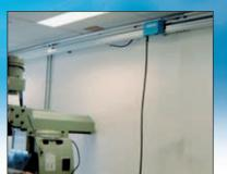
Pressurized pivoting arms in aluminium for feeding tools, covering a wide working radius. Swinging arms on benches, to support and feed pneumatic tools.
